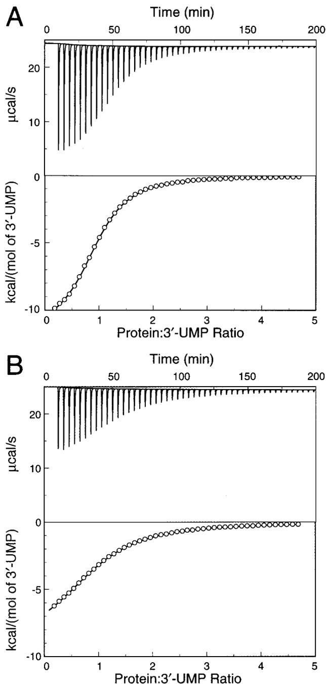
FIGURE 4: Thermograms for the binding of 3'-UMP to wild-type ribonuclease A (A) and K7A/R10A/K66A ribonuclease A (B) at 0.142 M Na<sup>+</sup>. The upper graphs show the heat released by the protein solutions upon injection of 3'-UMP. The lower graphs show the heat released upon binding versus the molar ratio of 3'-UMP to ribonuclease. Binding was measured by isothermal titration calorimetry at 25 °C in 0.10 M MES-NaOH buffer (pH 6.0) containing NaCl (0.10 M).
