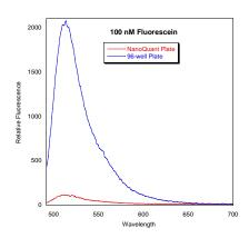
standard in 0.1 M NaOH. 96-well samples were run in triplicate and, following blank subtraction, could easily detect 1 nM fluorescein. NanoQuant samples were run in triplicate
